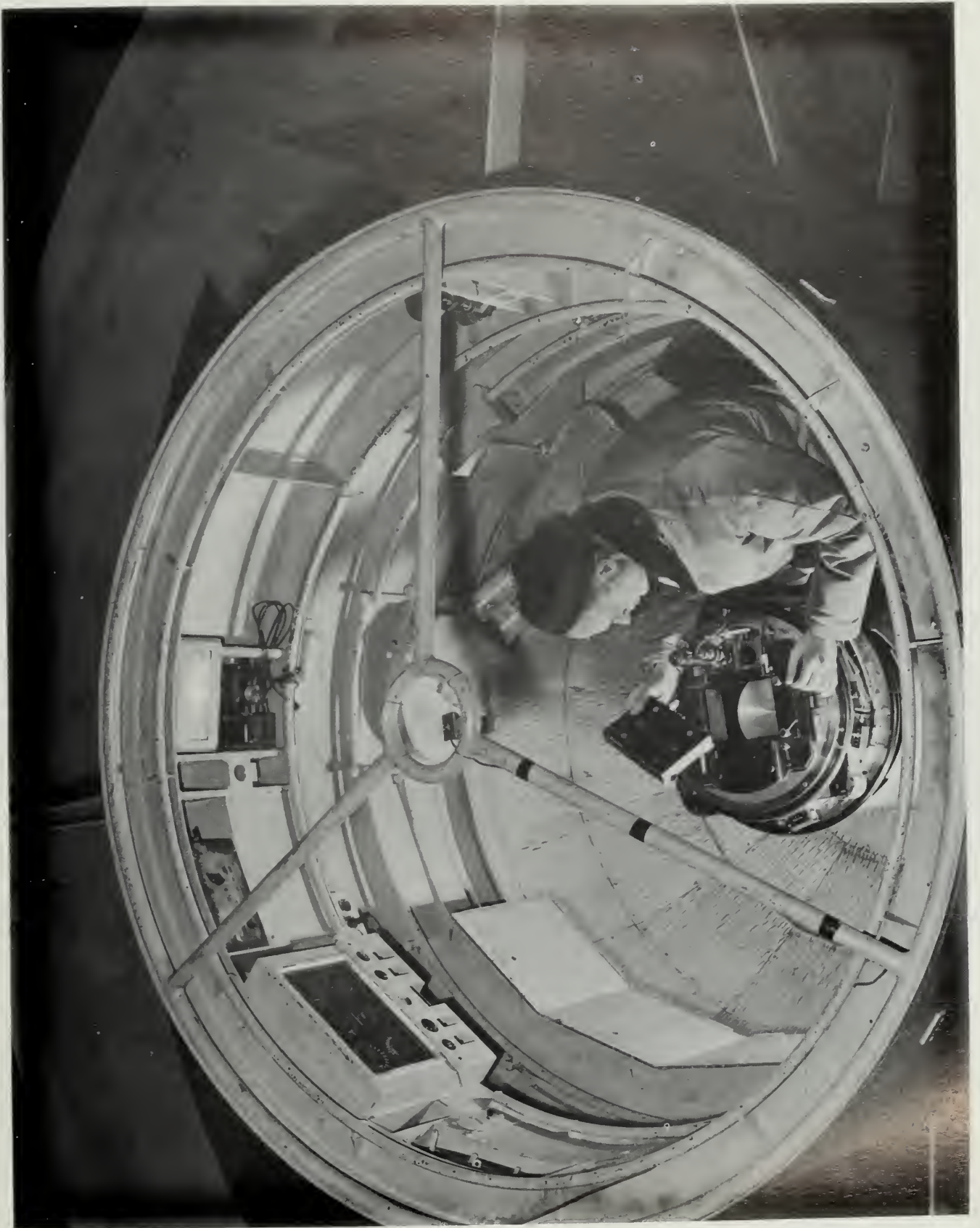
Palomar Observatory — San Diego County, California 200-inch Hale Telescope, showing the observer in prime-focus observing position, circa 1988
